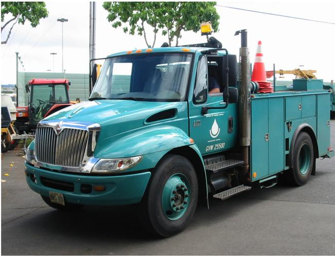
**Diesel Retrofits.** BWS trucks were retrofitted with devices that burn off and filter out much of the diesel particulate matter before discharging it.
