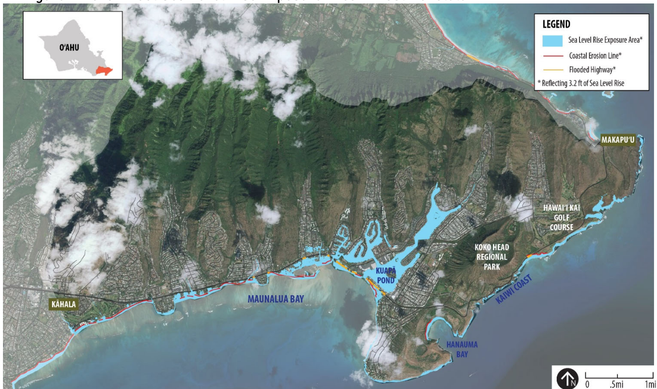
Figure 2-20: 3.2 Foot Sea Level Rise Exposure Area in East Honolulu
