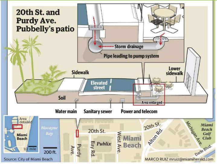
This rendering shows the elevated roadway at 20th Street and Purdy Avenue, in front of Pubbelly restaurant. To the right, the patio in front of Pubbelly is about two feet lower than the street. Floor drains down there feed into the same pipes that connect to the curb drains on the road, which routes water to the pump station.
