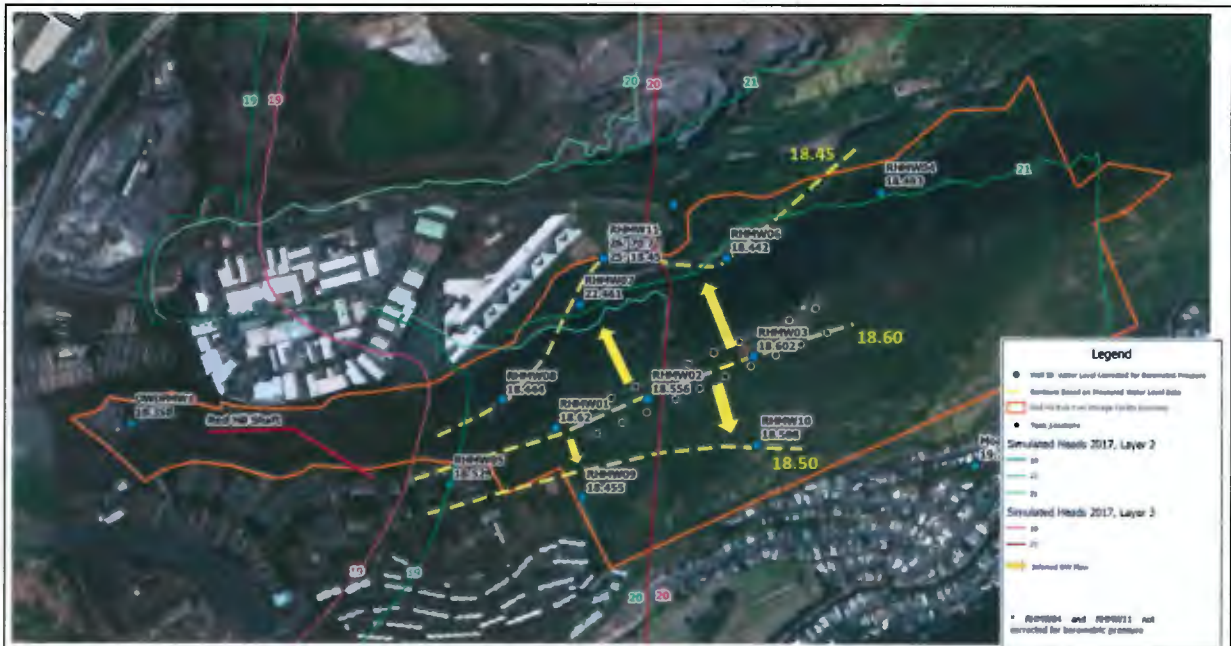
Figure 3 Measured water levels at 02/05/2018 19:00 after Red Hill Shaft has been pumping as usual and Halawa Shaft has not been pumping
