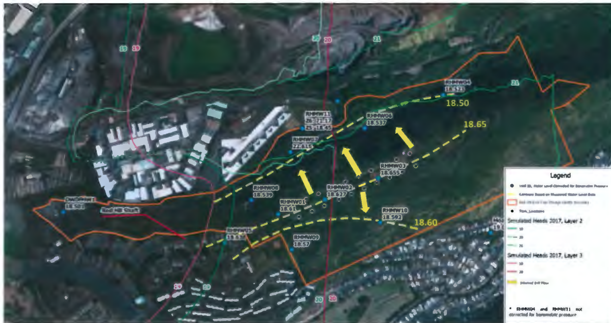
Figure 1 Measured water levels at 01/15/2018 6:00 after Red Hill Shaft has been not pumping for five days
