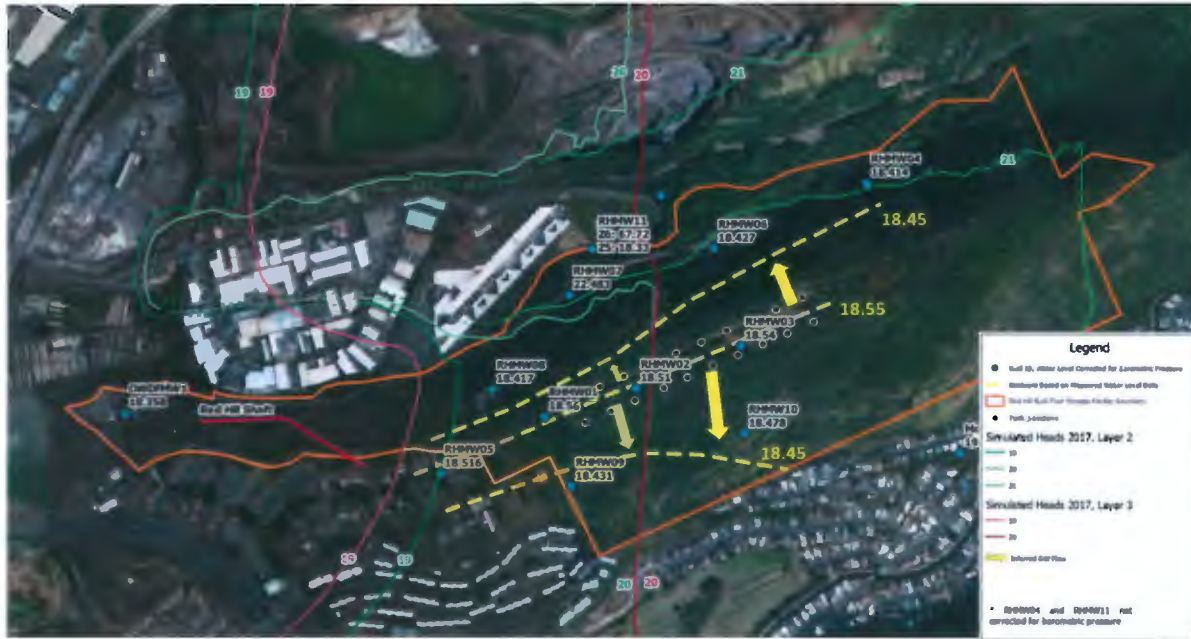
Figure 4 Measured water levels at 02/19/2018 13:00 after Red Hill Shaft has been pumping as usually and Halawa Shaft has maintained averaged pumping rate
