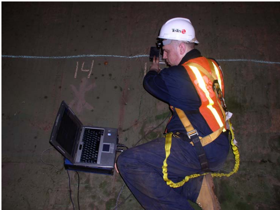
LFET scanning of course 2, quadrant A, of the lower dome.
