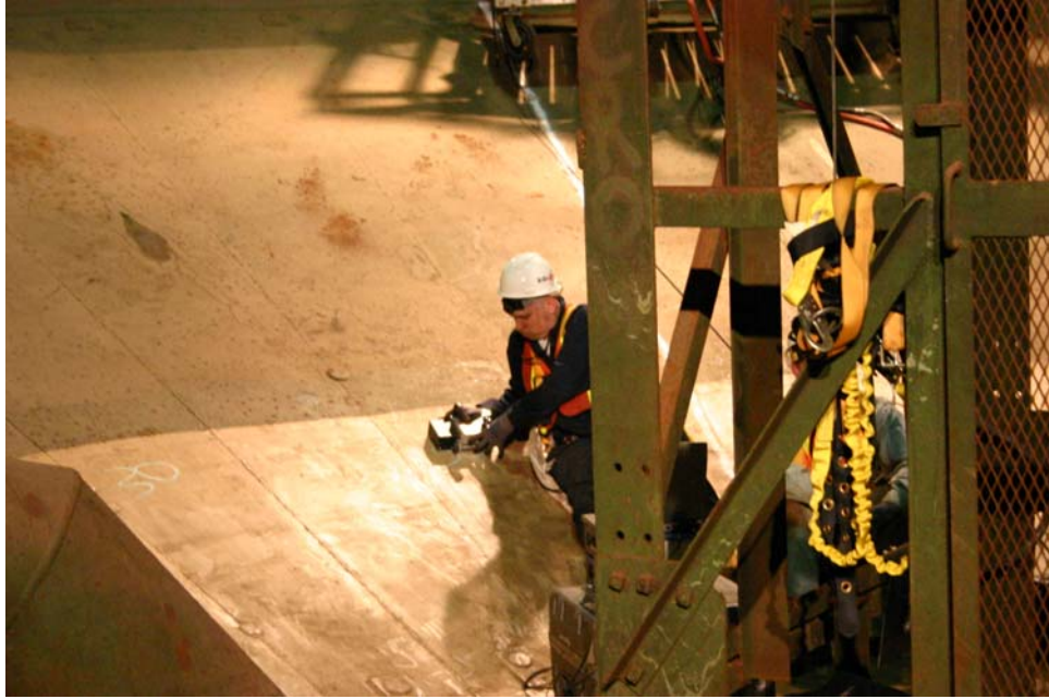
LFET scanning of course one, quadrant C, of the lower dome.
