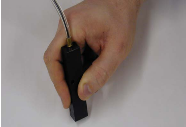
The Hawkeye Pencil Probe used for testing the welds of the floor, course 1, course 2, barrel, extension, and expansion of Tank # 6.
