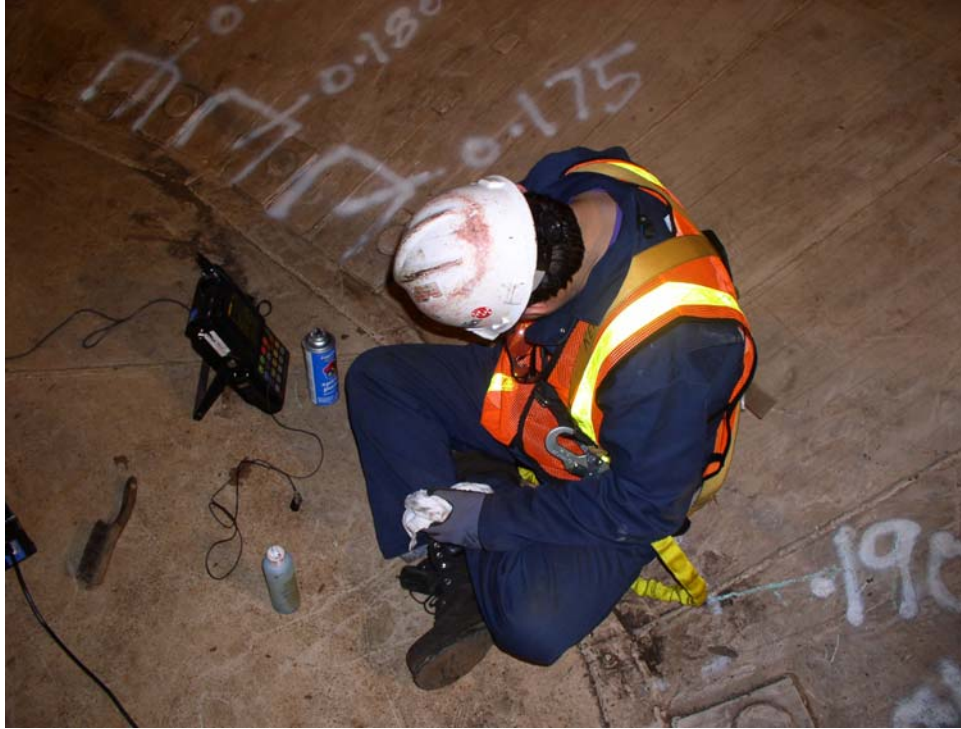
Shear wave U.T. measurements being taken at the interface between the floor and course one of the lower dome.
