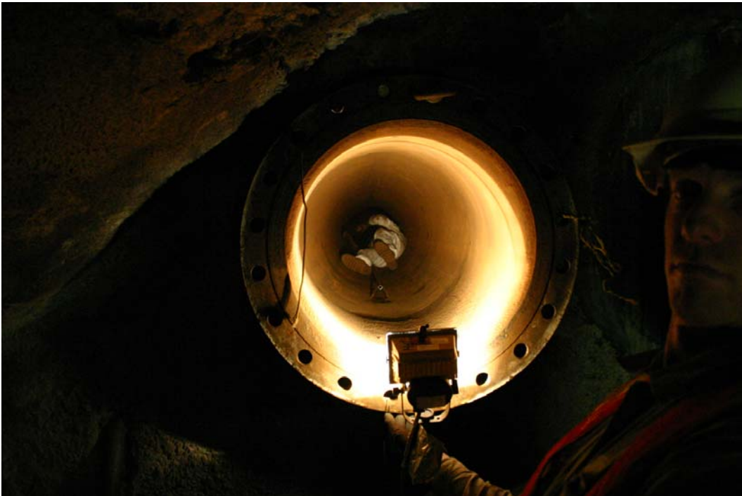
Photograph 10 – NDE technician/examiner taking UT measurements inside the 32” nozzle. Note the 3/4-inch pipe on the bottom of the nozzle.
